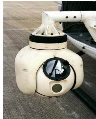
A forward looking infrared (FLIR) camera mounted on the side of an UAV
